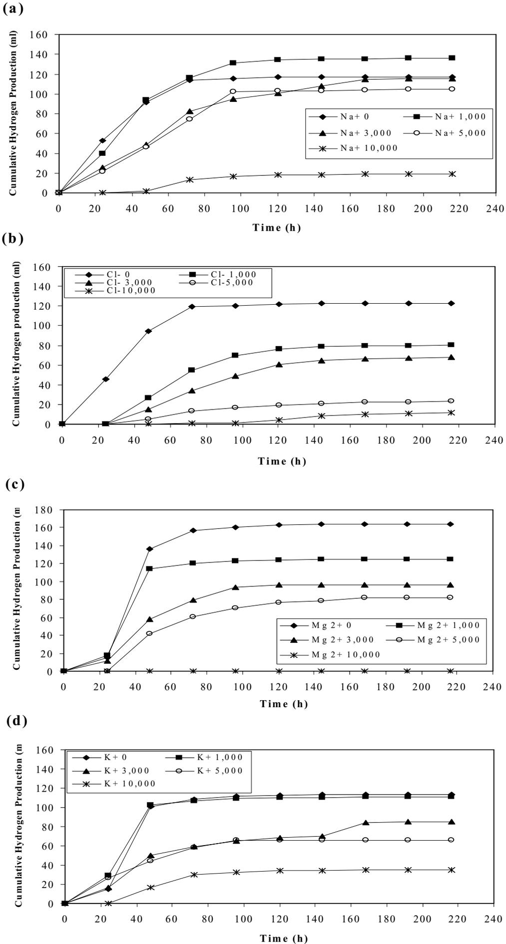
Figure 1. Hydrogen gas produced in batch tests with different ionic formulas and concentrations. (a) 0-10,000 mg Na<sup>+</sup> as NaHCO<sub>3</sub> mg/l (b) 0-10,000 mg Cl<sup>-</sup> as NaCl mg/l (c) 0-10,000 mg Mg<sup>2+</sup> as Mg(NO<sub>3</sub>)<sub>2</sub>·6H<sub>2</sub>O mg/l, and (d) 0-10,000 mg K<sup>+</sup> as K<sub>2</sub>CO<sub>3</sub> mg/l.
