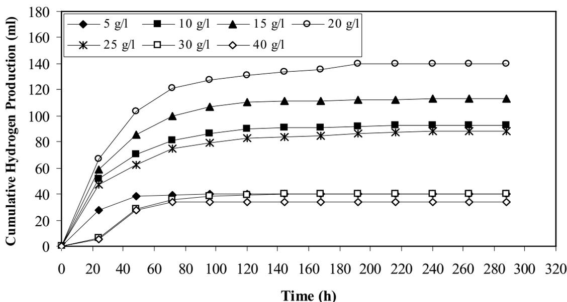
Figure 2. Effect of glucose concentrations on hydrogen production.
